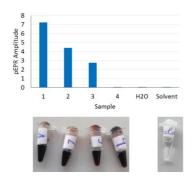
Sample 1,2,3,4: mixture of iron-salts and iron oxide nanoparticles Sample  $H_2O$  and Solvent: pure water and pure solvent
